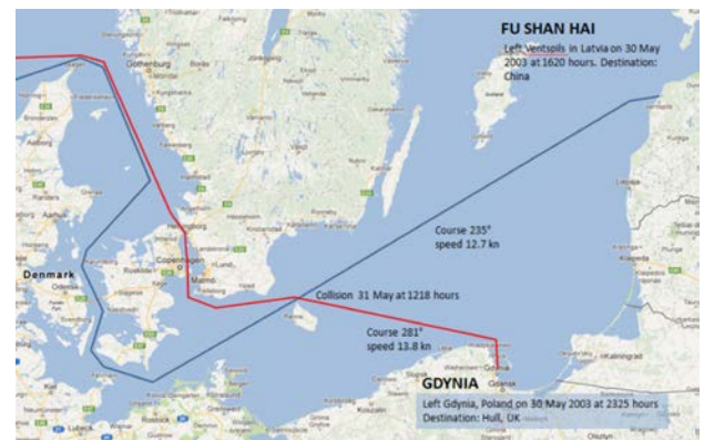
Figure 5: FU SHAN HAI and GDYNIA collided in open sea and good visibility 31 May 2003 [Adapted from 11].
