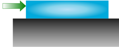
Figure 6 Schematic overview of the horizontal shear test, also called push test.
