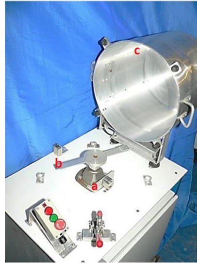
FIG. 2. The centrifuge adhesion test set-up with the centrifuge at position a, the iced beam at position b and the cover with the piezoelectric cells at position c.
