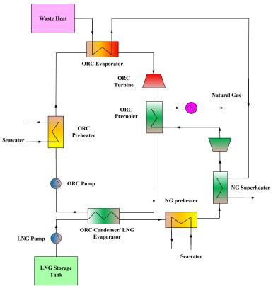
14 Fig. 2 The flowsheet of the Combined ORC and DE with Waste heat utilization (CODW)
