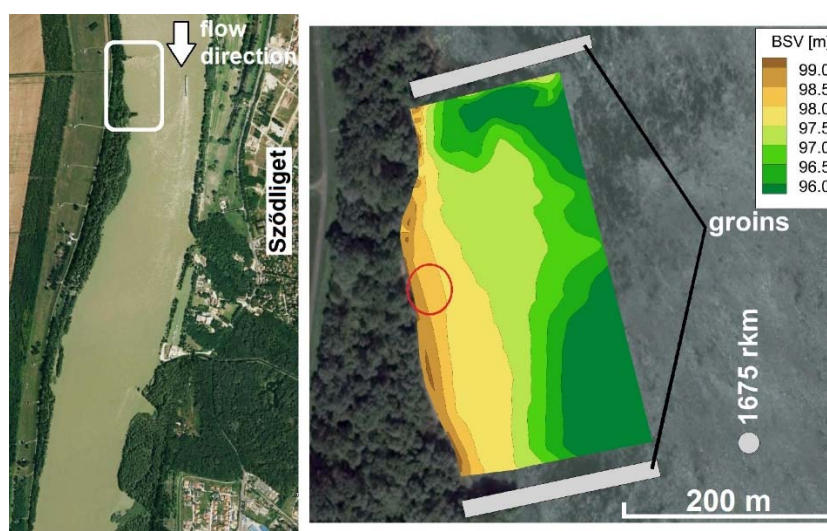
Figure 1. Ortophoto of the study site, marked with the white circle in the magnified right view. Bed elevation (meters above Baltic Sea) contour map is triangulated based on acoustic depth and GPS measurements. The mean water level during the measurements was 99.95 m.
