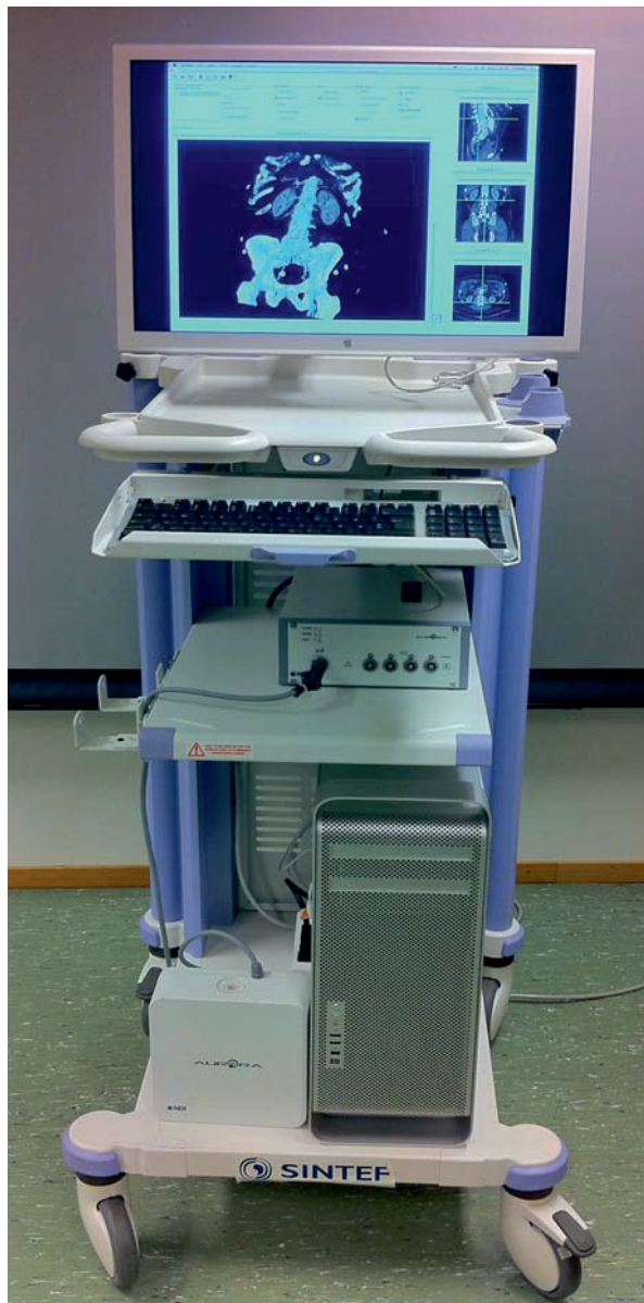
Figure 5. The in-house navigation system consists of a computer workstation on which the navigation software is installed, a navigation screen and a control unit. The navigation image can also be streamed to a larger, roof-mounted screen next to the operator in the operating room.
