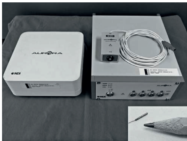
Figure 1 ♦ The electromagnetic (EM) field generator, control box, and position sensors. The EM field generator mounted underneath the operating table induced an EM field measuring \sim 0.5 \times 0.5 \times 0.5 m. The control box processed the data from the EM field generator and sensors and made it available to the navigation system. The position sensors measured 0.8 \times 11 mm and were embedded in the catheter tips. When a sensor was positioned within the EM field, a weak electrical current was induced, which enabled the tracking software to deduce the catheter's position along the x, y, and z axes.
