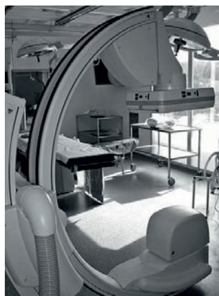
Figure 3 ♦ Cone-beam CT. The angiography suite was equipped with a ceiling-mounted Siemens AXIOM Artis dTA imaging system. Images were obtained consecutively and reconstructed into a CT volume as the C-arm rotated 270°.
