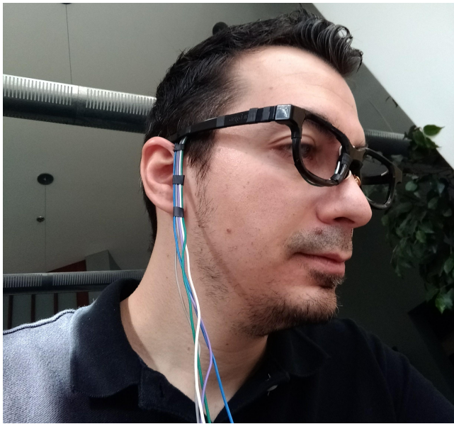
Figure 1: The EEGGlass prototype worn by a user.
