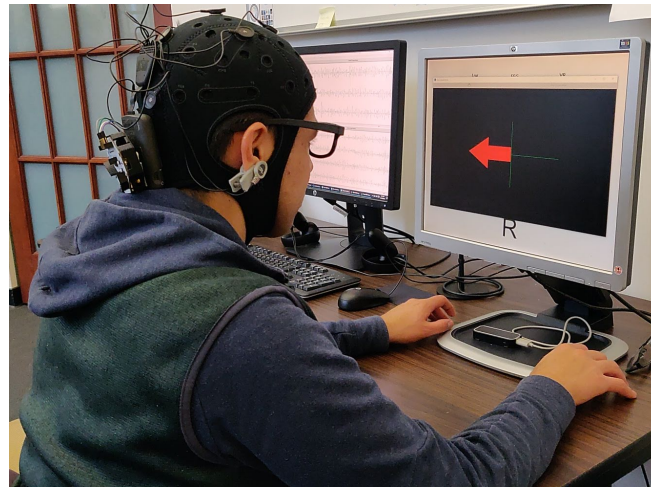
Figure 4: A user performing a motor task while wearing both EEGlasses and Enobio 8 EEG systems.
