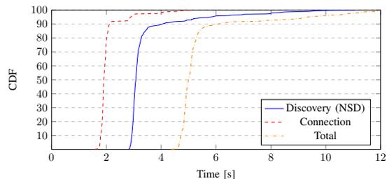
Fig. 5. CDF of the time to discover credentials over NSD and connect to a WiFi Direct group as a legacy client.
