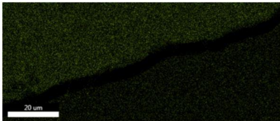
Figure A5.8: Mapping result showing the magnesium content of sample 2 from series 1 in area 3
