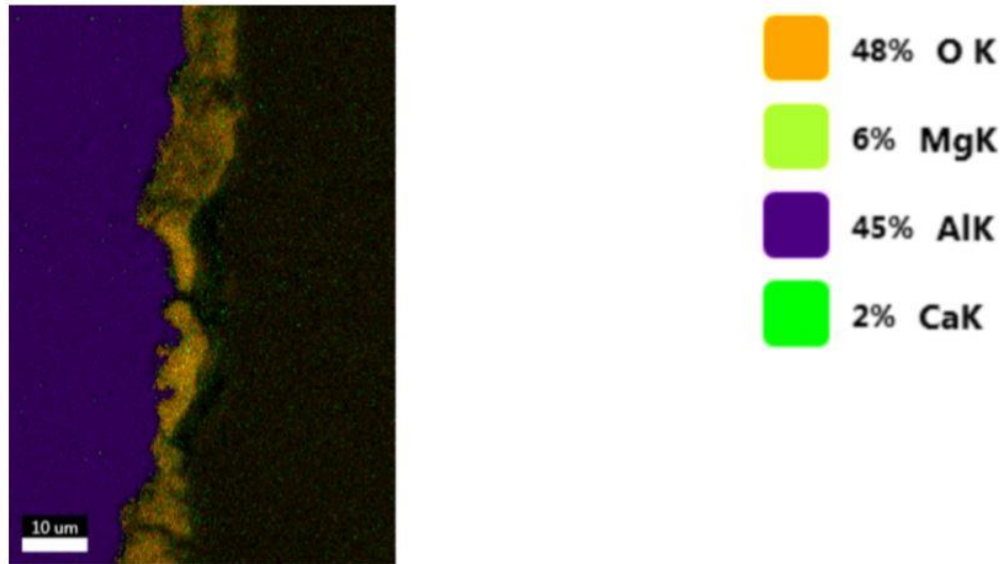
Figure A5.43: Element overlay from the cross section of sample 6 from series 3 in area 3. Sample not anodically polarized prior to inspection.
