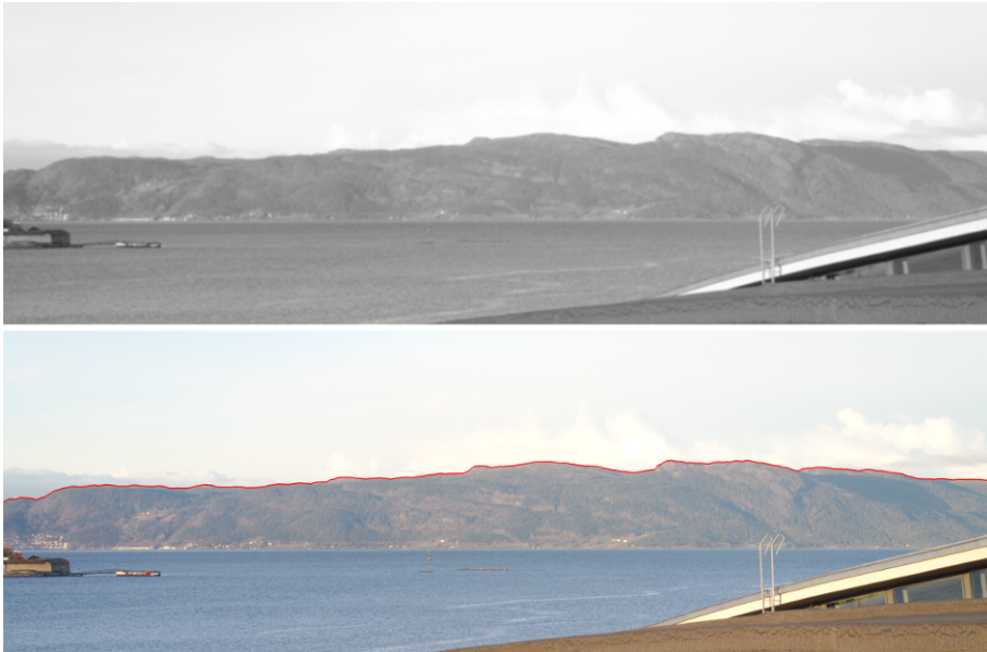
Figure 3.8: A sample camera image from the experiment. The top image shows the camera image converted to gray scale and with a Gaussian filter applied. The bottom image shows the camera image in its original color, with the camera skyline marked in red.
