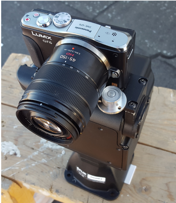
Figure 3.6: The camera system as mounted on the PTU in the experiment.
