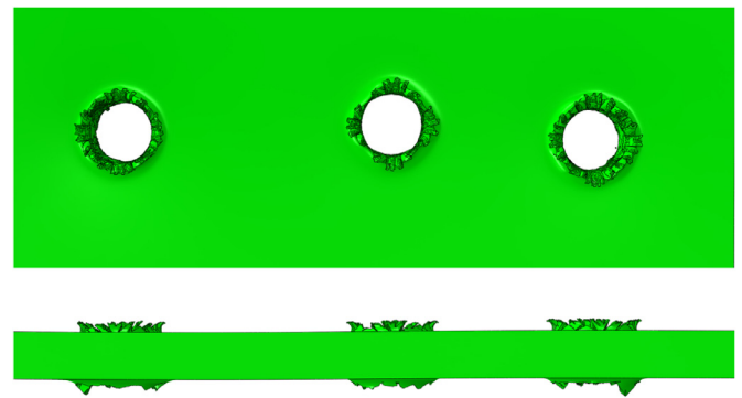
Fig. 22. Finite element simulation results of an AM plate perforated by three AP bullets seen from the front (top) and the side (bottom). Note that the images have been cropped to better show the details.
