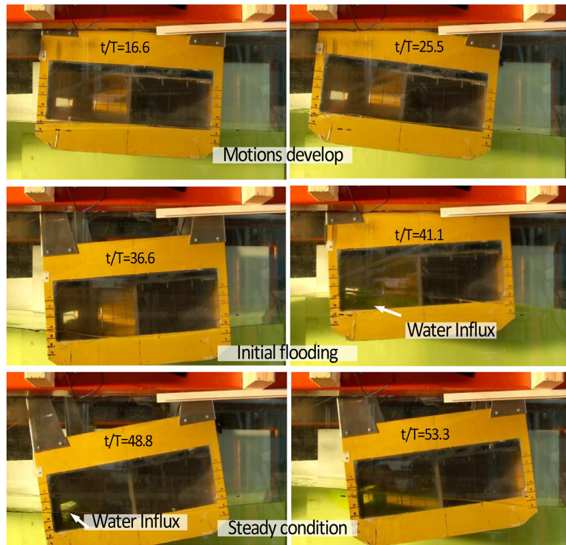
Fig. 34. Sequence of flooding as it occurs over time for the model in loading condition GM1 in waves with period T = 0.9 s and kA = 0.066 . Time increases from left to right and from top to bottom.
