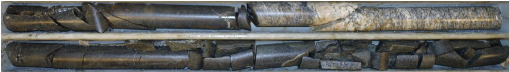
Fig. 10 Picture of a core section with heavily fractured amphibolite, each row of core represents 1 metre.
