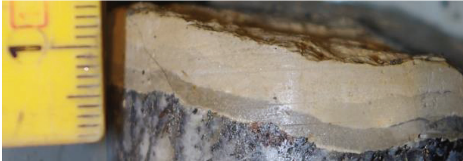
Figure 19: Picture of the drill core showing a subhorizontal cemented fracture with an approximate aperture of 8 mm. The cement appears to have 3 layers (Paper III).
