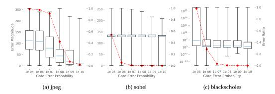
Fig. 11. Error magnitude (boxplots - left axis) and error ratio (lines - right axis) for the benchmark applications.
