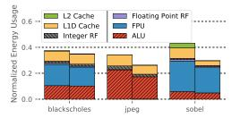
(b) Dynamic energy used by select components for precise (left) and approximate (right) execution, normalized to the total energy used by the precise CPU.
