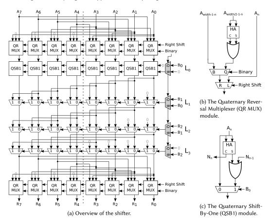
Fig. 5. A quaternary bidirectional shifter capable of operating with both quaternary and binary data. The gates shaded gray are binary gates, while the rest are quaternary.
