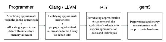
Fig. 10. The process used for evaluating the proposed quaternary hardware with benchmark applications.
