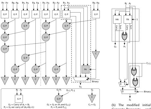
(a) Overview of the adder circuit. The part of the figure indicated with the dashed outline is depicted in more detail in Fig. 3b.
