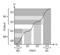
Fig. 1. Illustration of a quaternary device that can operate on binary data. Gray regions represent the input and output ranges when working with quaternary data. Striped regions represent input and output ranges when working with binary data. The figure is explained in more detail in Sec. 3.
