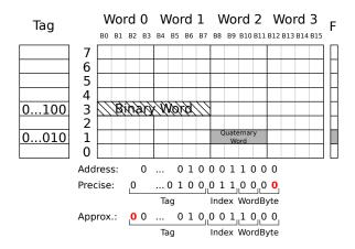
Fig. 6. A direct mapped cache that can store both binary and quaternary data. The shaded cells represent the word that the address points to. While the figure depicts a direct mapped cache, additional ways can be added without any design modifications.
