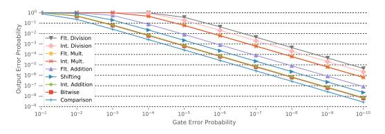
Fig. 8. The probability of an error appearing in the output of a circuit, given the probability of an error occurring in a gate.
