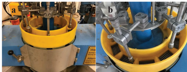
Figure 13: Details from the pilot WHIMS. The magnetic pole pieces are the blue blocks on either side (a). The measurements, with the Gauss-meter, were conducted inside the grooves at the position of the flushing and feed tubes (b).
