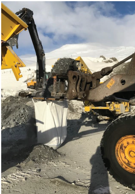
Figure 7: The sampling of the conveyer belt from the mobile jaw crusher by wheel loader with big-bag. Each sample was collected at 3x10 sec intervals. The entire width of the stream was sampled.
