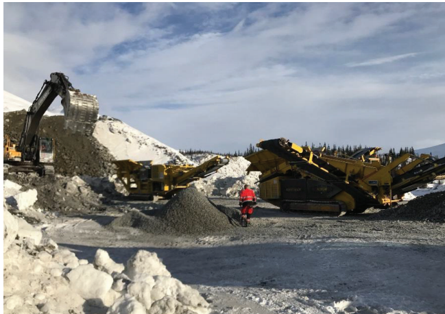
Figure 6: The mobile jaw crusher used to crush the sampled blast from the Kvannevann deposit.
