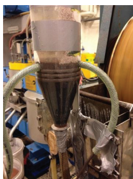
Figure 12: The “Mozell”-splitter, constructed on site, was placed on the LIMS feed.
