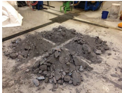
Figure 8: The crusher output from Kvannevang 1 deposit sample during the quartering to get a representative split for PSD analysis. This was repeated for the crusher output from the Kvannevang 2, Stensundtjern, and Stortjønna deposit samples.
