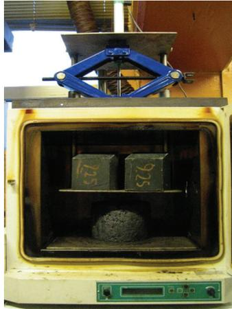
Figure 4-4: The furnace for flow measurements with sample inside.
