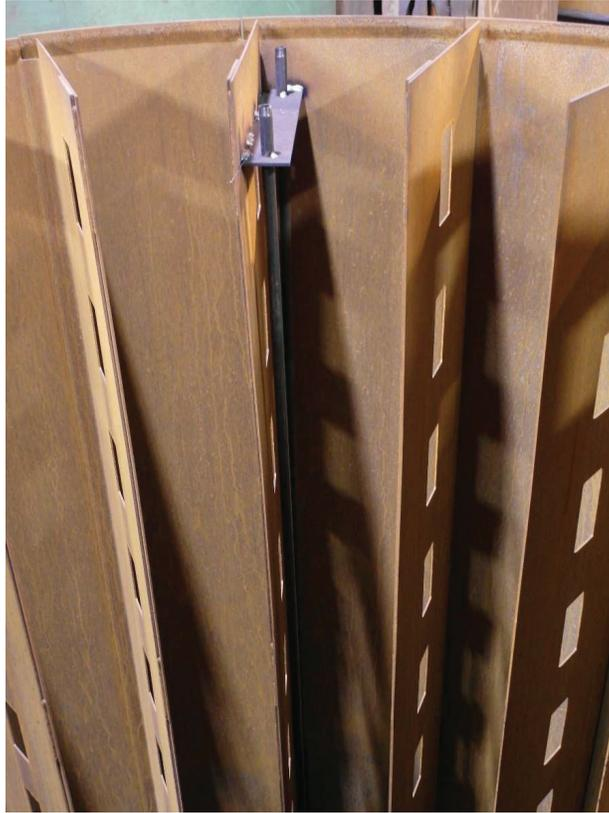
*Figure 3-6: The steel tubes for thermocouples 7 and 8 attached to the fin of the electrode casing*
