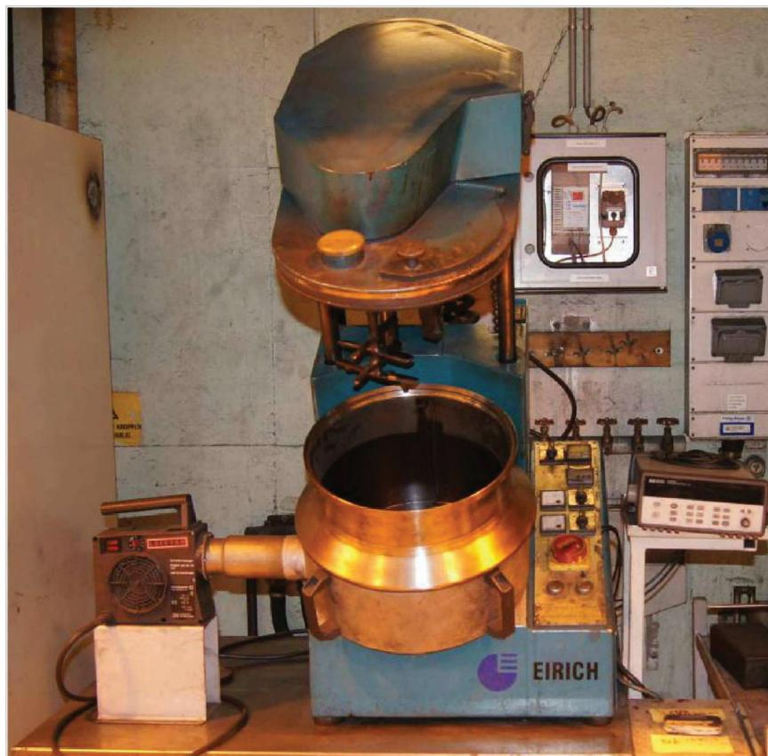
Figure 4-3: The Eirich high intensity mixer used to prepare electrode paste.
