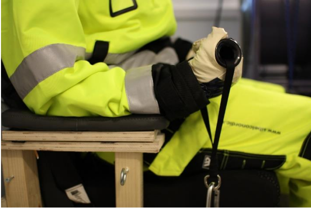
Fig. 3. Right wrist flexion MVC. Arm resting on an armrest, elbow angle in approximately 90° and forearm supinated. The same position was also applied for DWF.
