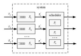
Fig. 4. The system architecture with shapers
