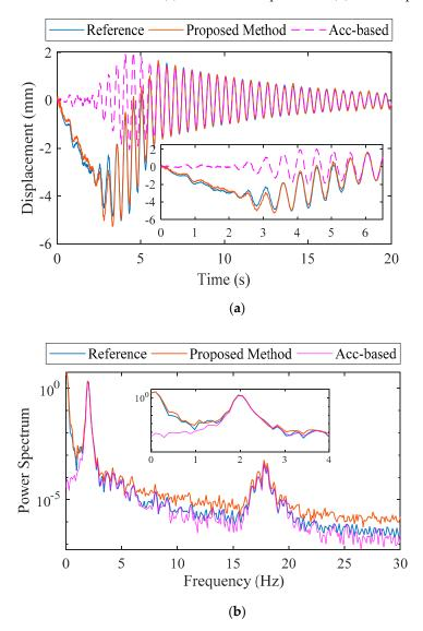
Figure 5. Numerical validation: (a) estimated displacement and (b) frequency response.
