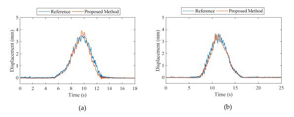
**Figure 8.** Comparison of maximum displacements at the mid-span point of the bridge: (**a**) truck speed of 5 km/h (**b**) truck speed of 15 km/h.
