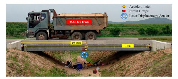
Figure 7. Experimental setup for field validation.
