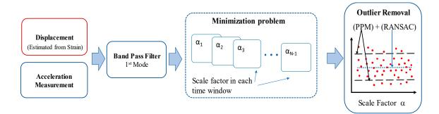
Figure 2. Overview of calibration factor estimation.
