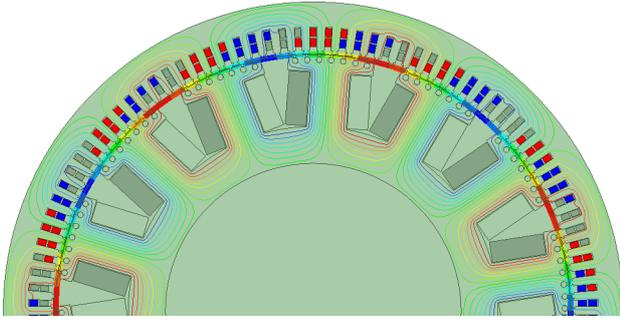
Fig. 1. 2-D modeling of SPSG using FEM
