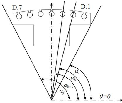
Fig. 2. Rotor pole and location of damper bars of SPSG
