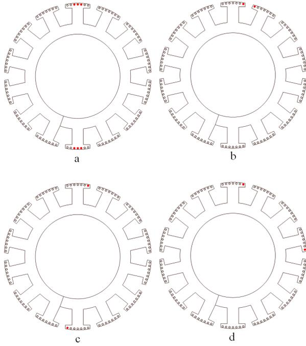
Fig. 5. Location of broken damper bars of the SPSG, (a) six BDBs in each opposite poles, (b) two BDBs in the edge of two adjacent poles, (c) two BDBs in the edge of two opposite poles, (d) two BDBs at two-pole pitch distance.
