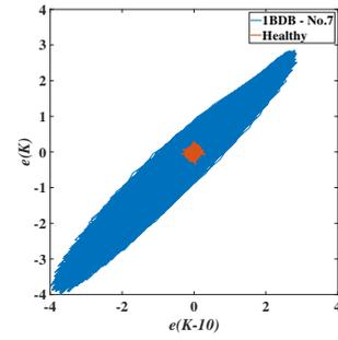
Fig. 4. Phase space of the healthy and one broken damper bar at the edge of SPSG rotor pole.
