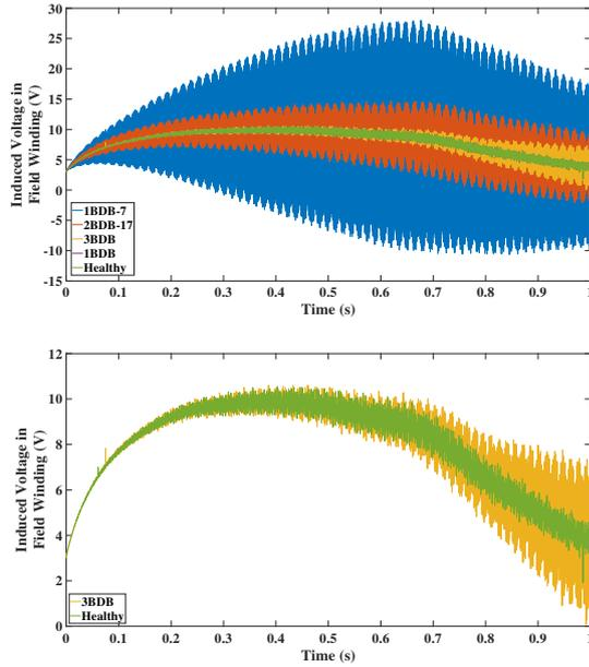
Fig. 3. Induced voltage in the rotor field winding of a SPSG in the healthy, and faulty cases for different number of BDBs.
