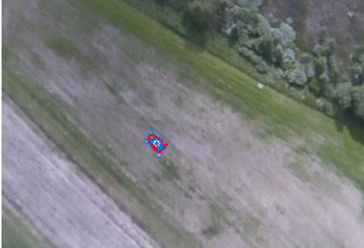
Figure 4.14: The resulting processed image with the detection marked. The red areas mark the detected contours and the white circle marks the center of detection that is used for georeferencing.
