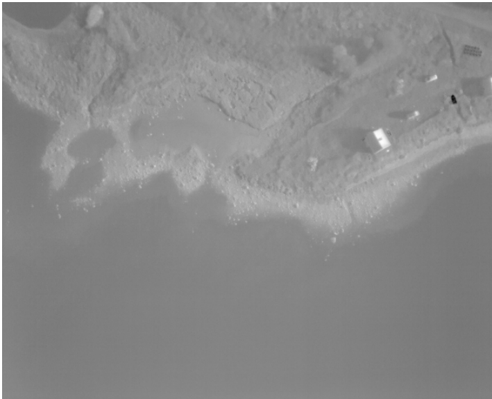
Figure 2.2: Example of image in the long wave infrared spectrum captured with a thermal camera. The image shows areas with sea, land, two buildings and a couple of cars. The emissivity of the ground is stronger than the emissivity of the sea surface and explains why it is possible to observe where the sea surface ends.
