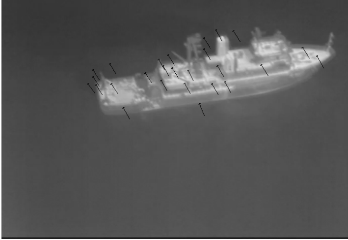
Figure 4.2: Optical flow (arrows) and features (arrow origin) in a thermal image at sea
