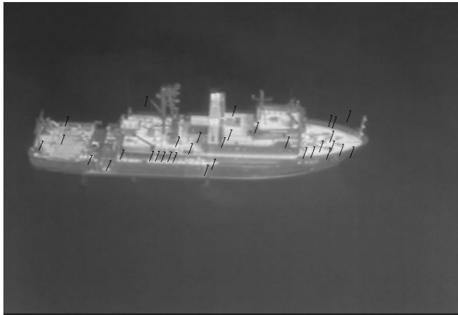
Figure 5.13: The large vessel used in the third case study with optical flow vectors
