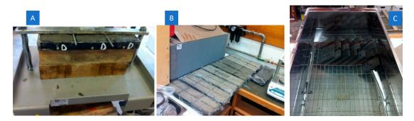
Figure 5. (A) Compacting pastes at shaking table, (B) initial 24-h air curing and (C) water curing thereafter.
