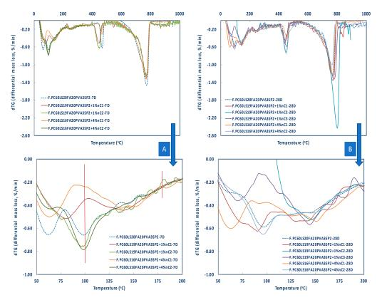
**Figure 9.** Differential mass loss between 100–200 °C of nMt and fibre reinforced cementitious nanocomposites at (**A**) Day 7 and (**B**) Day 28.
