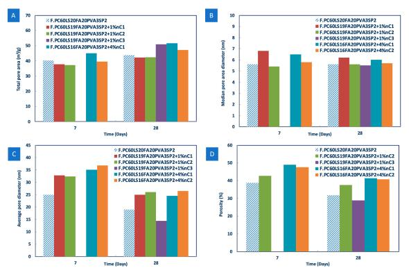
**Figure 15.** Effect of nMt type on (**A**) the total pore area, (**B**) the median pore area diameter, (**C**) the average pore diameter and (**D**) the porosity of fibre cements.
