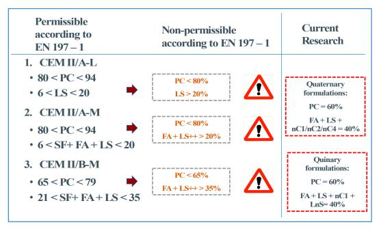
**Figure 2.** Eurocode limits of clinker substitution and supplementary cementitious materials (SCM) addition and target of current research.
