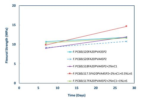
**Figure 7.** Flexural strength of nC1 and nanosilica (LnS) and fibre reinforced cementitious nanocomposites based on F.PC60LS20FA20PVA4SP2.
