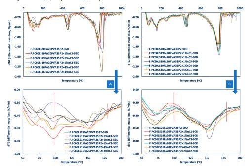
**Figure 10.** Differential mass loss between 100–200 °C of nMt and fibre reinforced cementitious nanocomposites at (**A**) Day 56 and (**B**) Day 90.
