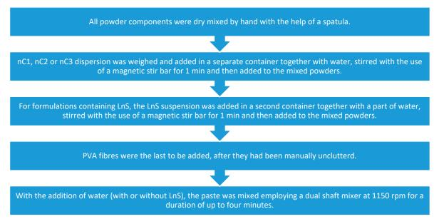
Figure 3. Flow chart of the mixing procedure.
