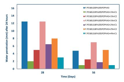
**Figure 16.** Effect of nMt type and concentration on the impermeability of nMt and fibre reinforced cementitious nanocomposites based on F.PC60LS20FA20PVA3SP2.
