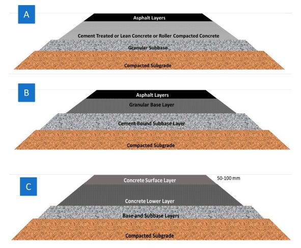
Figure 1. Cross sections of (A) a semi- rigid pavement, (B) an inverted pavement and (C) composite two-lift pavement [21].
