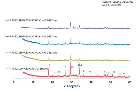
**Figure 12.** XRD pattern of 1% nMt and fibre reinforced cementitious nanocomposites at day 28—Effect of nMt type.
