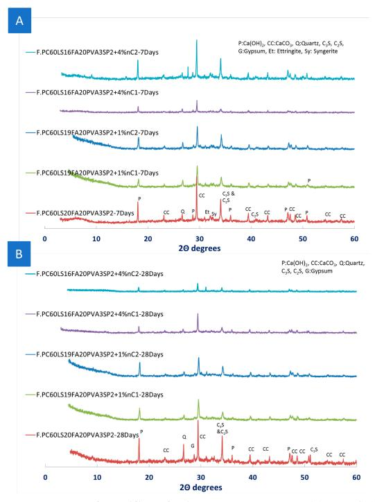
**Figure 11.** XRD pattern of nMt and fibre reinforced cementitious nanocomposites at (**A**) Day 7 and (**B**) at Day 28—Effect of nC content and type.
