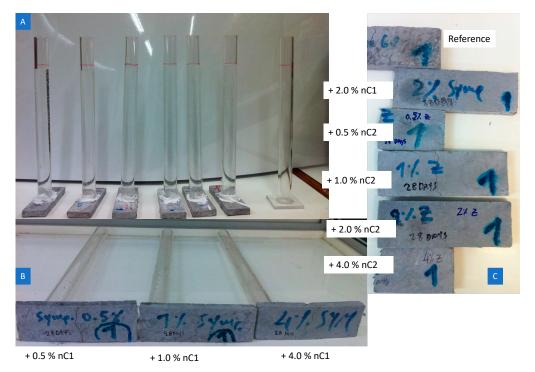
**Figure 17.** (**A**) Example of impermeability test, (**B**) difference in water absorption between the various concentrations of the nC1 and fibre reinforced cementitious nanocomposites and (**C**) difference in water absorption between the various concentrations of the nC2 and fibre reinforced cementitious nanocomposites based on F.PC60LS20FA20PVA3SP2.
