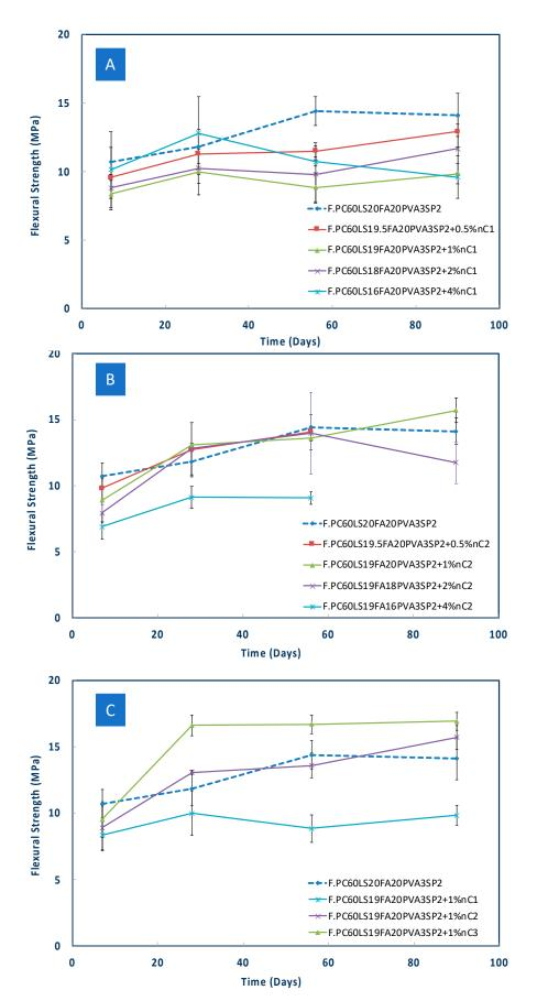
**Figure 6.** Flexural strength of (**A**) nC1, (**B**) nC2 fibre reinforced cementitious nanocomposites based on F.PC60LS20FA20PVA3SP2 (**C**) comparison of flexural strength of 1% nC1, nC2 and nC3 fibre reinforced cementitious nanocomposites.
