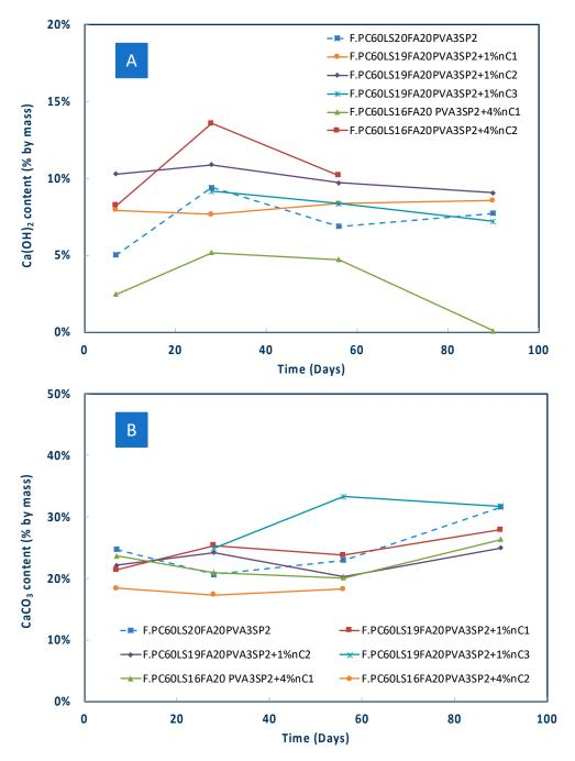
**Figure 8.** Effect of nMt content and type on (**A**) Ca(OH)<sub>2</sub> and (**B**) CaCO<sub>3</sub> content of nMt and fibre reinforced cementitious nanocomposites based on F.PC60LS20FA20PVA3SP2.
