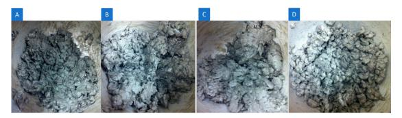
Figure 4. (A) 0%, (B) 0.5%, (C) 1% and (D) 4% by mass addition of nC2 on F.PC60LS20FA20PVA3SP2.
