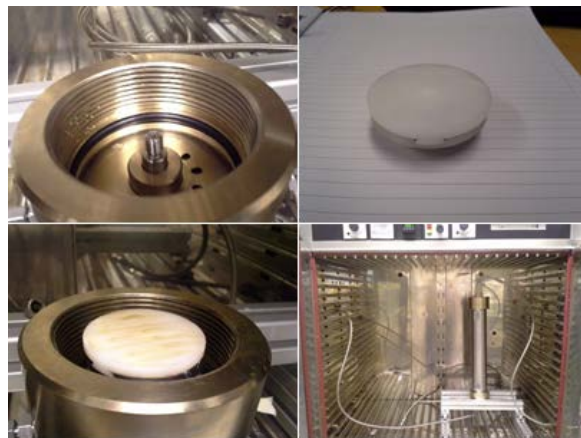
Figure 2 Photographs of test cell. Top left: bottom cap with teflon piston removed. Top right: teflon piston. Bottom left: bottom cap with teflon piston mounted. Bottom right: Fully assembled test setup inside heating cabinet.
