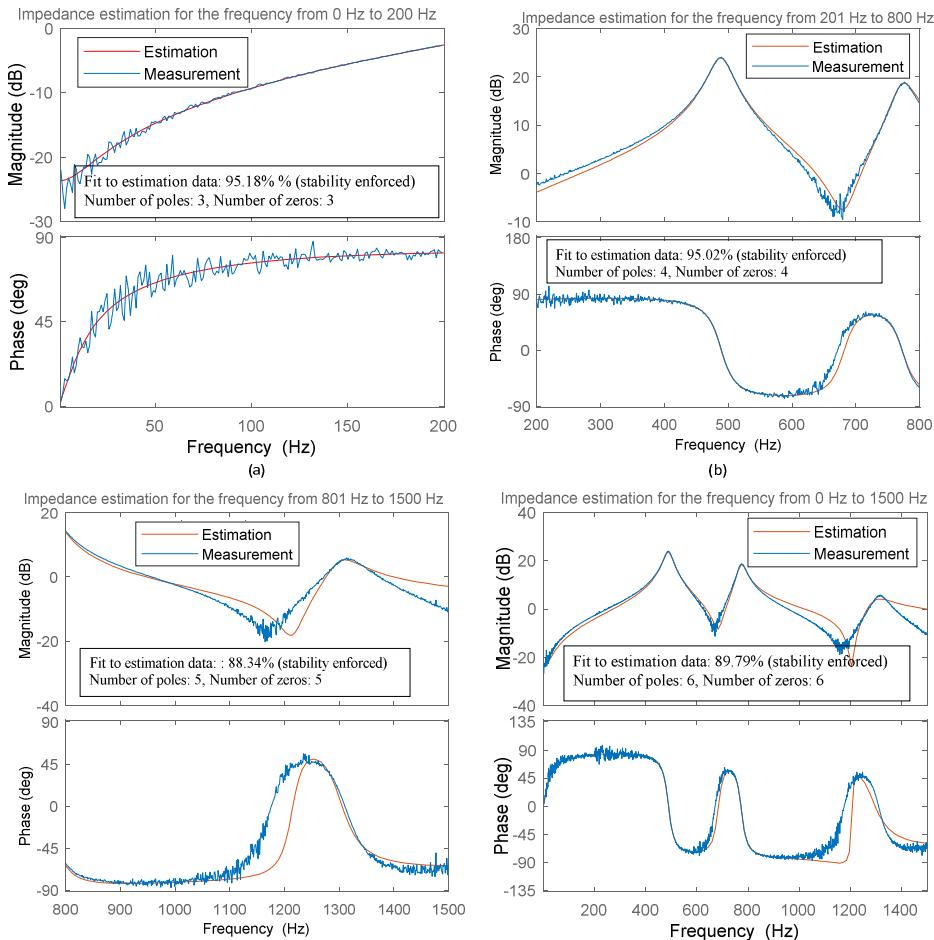
Figure 5. Grid impedance identification results
