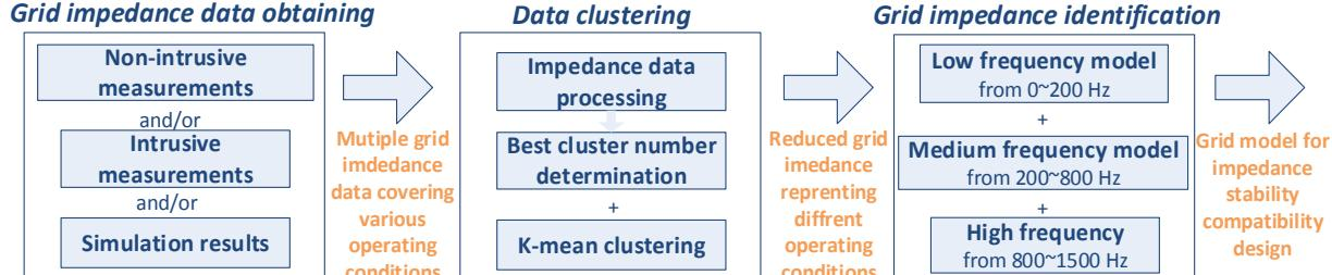
Figure 1. Flowchart of proposed data-driven approach for grid impedance identification
