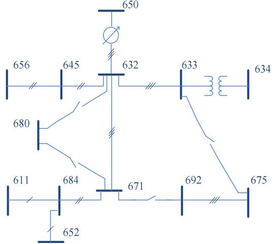
Figure 2. IEEE 13-bus test feeder with two added transmission lines
