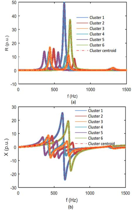
Figure 4. Grid impedance data partition results
