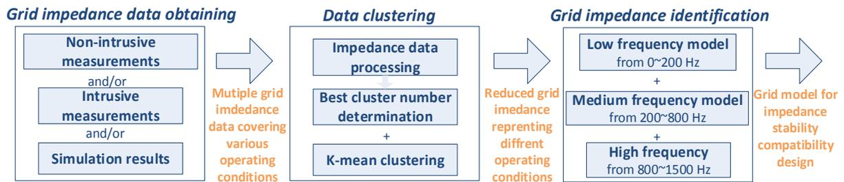
Figure 1. Flowchart of proposed data-driven approach for grid impedance identification
