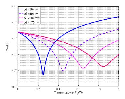
Figure 3. The Nash equilibrium of the D2D user depends on the transmit power of the cellular user.
