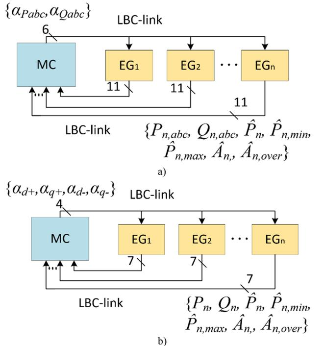
Fig. 1. Communication in the a) conventional and b) proposed PBC.
