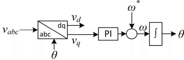
Fig. 2. Controller Phase-Locked Loop.
