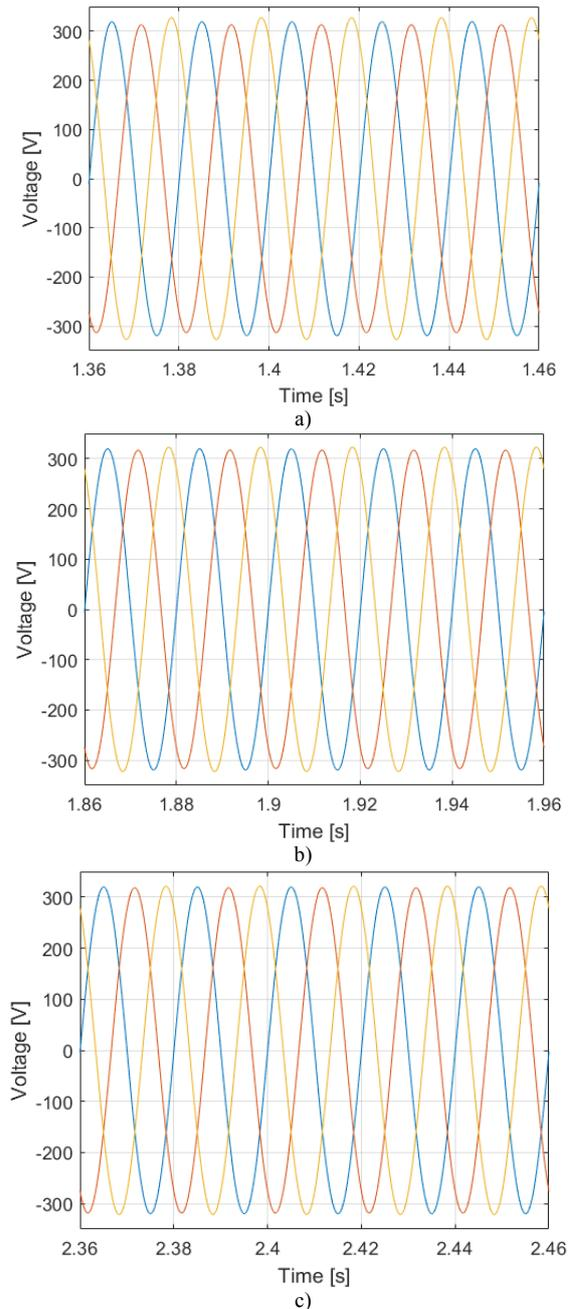
Fig. 7. Load voltages under a) the original PBC, b) the proposed PBC and c) the proposed PBC with weighting factor.
