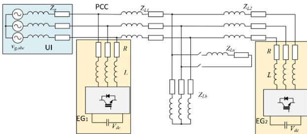
Fig. 5. Simulation setup of the test microgrid.
