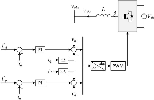
Fig. 4. Structure of EG current controller.
