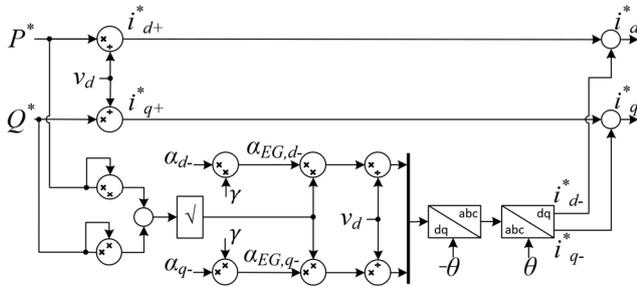
Fig. 3. Structure of EG power controller.
