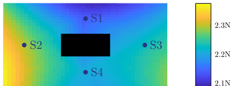
Fig. 5. Sensor interface pressure. The force distribution is estimated by linear interpolation of the mean forces of each of the force signals presented in Fig. 3.
