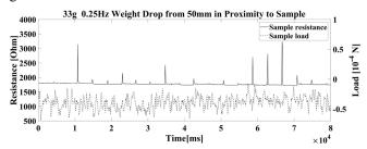
Fig. 2. Peaks of increasing resitance as a weight is dropped on a wooden table top in proximity to the sample every four seconds. The non-uniform weight shape might explain the differences in resistance change as the weight disperses its energy differently depending on its orientation upon impact.
