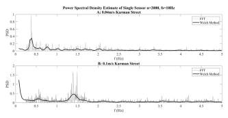
Fig. 4. Power spectral density analysis of single sensor. The shedding frequency for A was observed to be 0.58Hz, while the shedding frequency for B was observed to be 1.5Hz. Peaks in both plots are in proximity to their expected shedding frequency.
