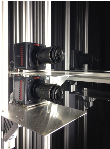
Figure 4.8: Camera setup with two Photron FASTCAM Mini AX100 540K M3 cameras mounted to metal shelves.
