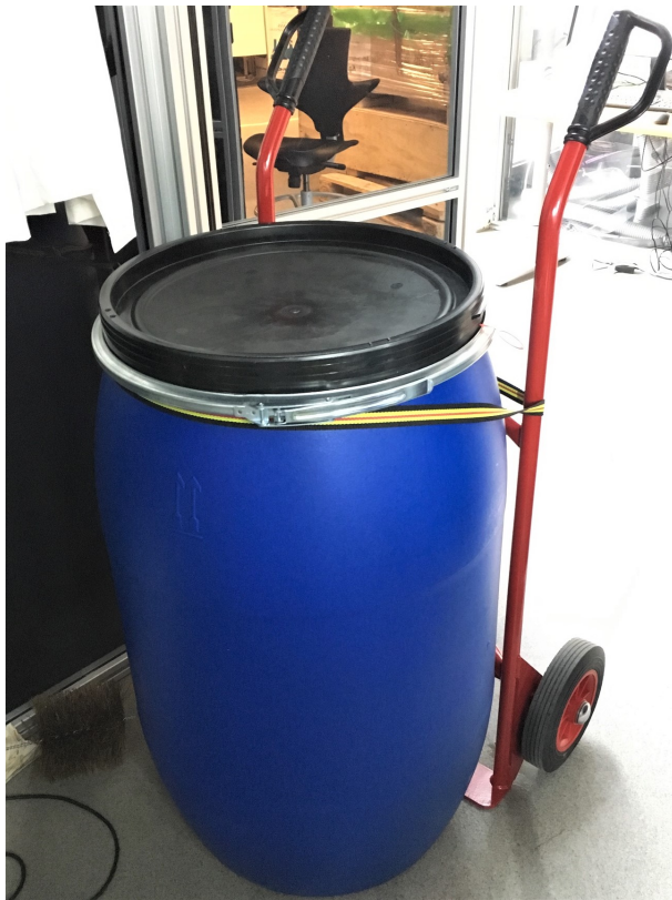
Figure A.2: Plastic containers used for storage of de-ionized water before emptying and refilling the water reservoir tank in the experimental apparatus.
