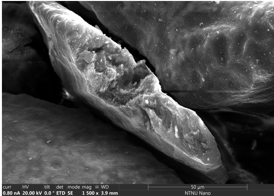
Figure 4.31: Surface morphology of MCS400 sample at 50µm magnification using a voltage of 20kV and a current of 0.80nA
