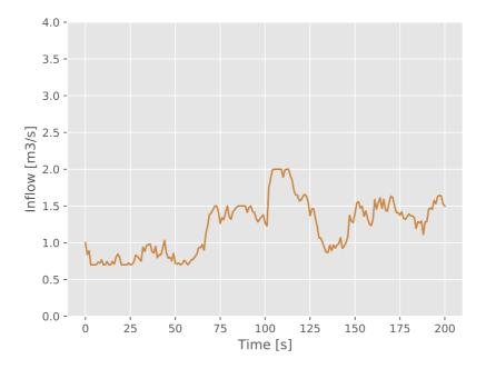
Figure 15: Predetermined inflow disturbance to be used in evaluation of controllers
