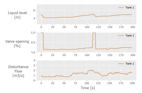
Figure 36: Evaluation of A2C-controller for the one tank case
