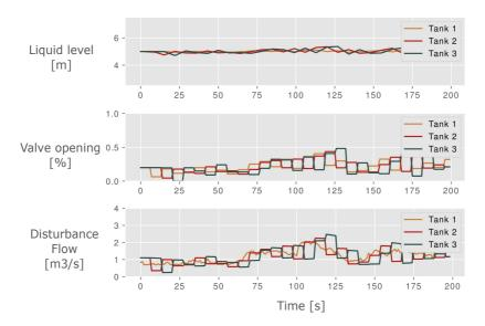
Figure 50: P-controller for six tank evaluation plot for the first three tanks with the  $\tau_c$  parameters calculated using the tuning script
