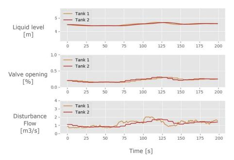
Figure 37: Evaluation of P-controllers for the two tank case
