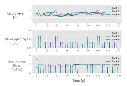
Figure 43: Evaluation of DQN-controllers of the last three tanks for the six tank case
