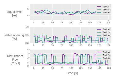
Figure 45: Evaluation of REINFORCE-controllers of the last three tanks for the six tank case
