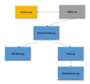
Figure 18: The overall python project structure of the tank system simulator
