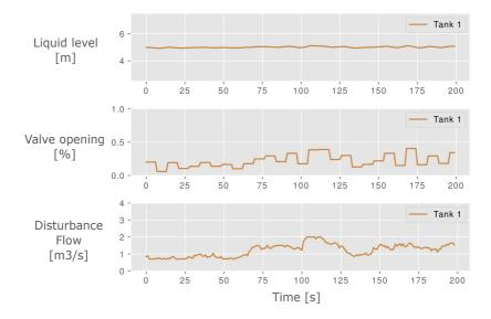
Figure 48: P-controller control for one tank evaluation plot with the  $\tau_c$  parameters calculated using the tuning script
