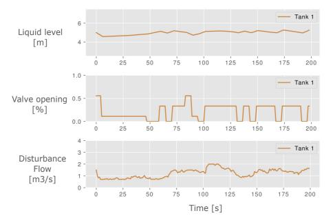
Figure 34: Evaluation of DQN-controller for the one tank case
