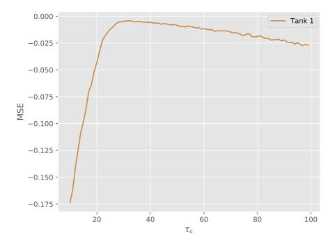
Figure 20: Error function evaluation of the p-controllers tuning parameters  $\tau_c$  for the first tank
