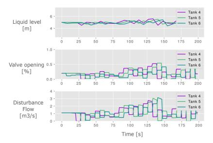
Figure 51: P-controller for six tank evaluation plot for the last three tanks with the  $\tau_c$  parameters calculated using the tuning script
