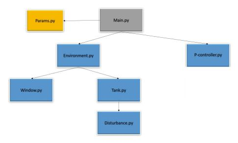
Figure 19: The overall python project structure of the p-controller implementation
