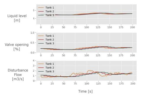
Figure 40: Evaluation of P-controllers of the first three tanks for the six tank case
