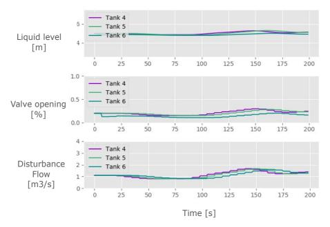
Figure 41: Evaluation of P-controllers of the last three tanks for the six tank case
