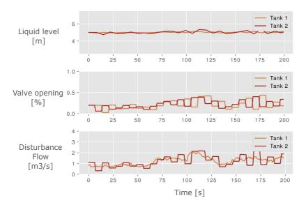
Figure 49: P-controller for two tank evaluation plot with the  $\tau_c$  parameters calculated using the tuning script
