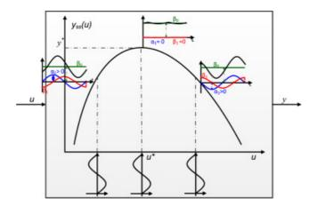
Figure 2: Illustration of the input value adjustment for increased performance for an extremum seeking adaptive controller. Figure aquired from Atta, Khalid Tourkey and Johansson, Andreas and Gustafsson, Thomas Extremum seeking control based on phasor estimation [11]
