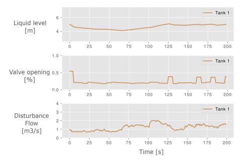
Figure 35: Evaluation of REINFORCE-controller for the one tank case
