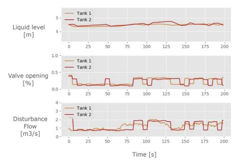
Figure 39: Evaluation of REINFORCE-controllers for the two tank case
