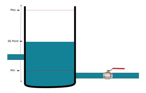
Figure 14: Illustration of a tank containing liquid with one disturbance inflow and one outflow with a choke valve
