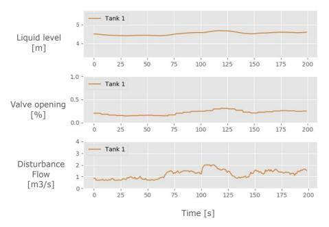
Figure 33: Evaluation of P-controller controller for the one tank case
