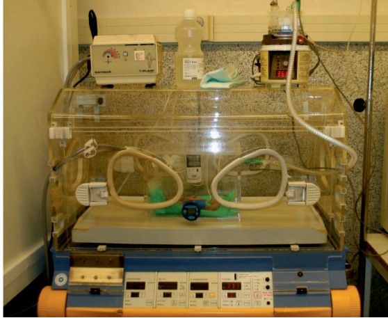
Figure 3 Hypoxia fibreglass box with rat pups inside a neonatal incubator with heated and humidified environment. Animals are atop of a water-heated bed, and the air of the box holds a temperature of 36 \pm 0.5 °C. The box is flushed with humidified and heated gas.
