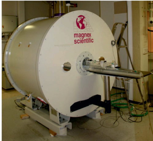
Figure 6 The 7 Tesla magnet (Biospec 70/20) utilized for longitudinal in vivo MR imaging of rats with designated animal bed.
