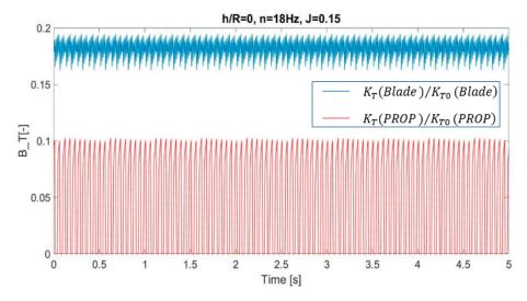
**Figure 19.** Time series of the computed thrust coefficient for a single blade and the propeller for J = 0.15, h/R = 0, n = 18 Hz,  $K_T(Blade)/K_{T0}(Blade)$  is the thrust loss coefficient for a single blade and  $K_T(PROP)/K_{T0}(PROP)$  is the thrust loss coefficient for the whole propeller.
