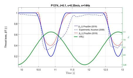
**Figure 3.** Comparison of thrust loss between simulation performed by using the PropSim (2016) simulation model, PropSim (2018) simulation model, and experimental results of *Kou 2006\_I*, the sampling rate is above four times the propeller revolutions, and it is equal to 60 Hz.
