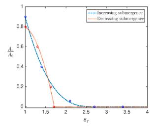
**Figure 2.** Ratio of ventilated propeller disk area to nominal disk area as function of propeller submergences ratios  $S_r$ , Dalheim [14]. Submergence ratio is denoted by the symbol  $S_r$ .
