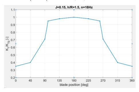
**Figure 12.** Calculation of thrust loss factor as a function of blade position using the simulation model PropSim (2018\_blade\_dynamics).
