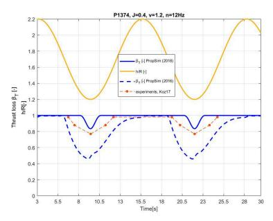
**Figure 4.** Comparison of thrust loss between the simulation performed by Dalheim (PropSim(2016)) and Kozlowska (PropSim (2018)) and experimental results of *Koz17*.
