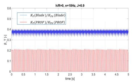
**Figure 20.** Time series of the computed thrust coefficient for a single blade and the propeller for J = 0.9, h/R = 0, n = 18 Hz,  $K_T(Blade)/K_{T0}(Blade)$  is the thrust loss coefficient for a single blade, and  $K_T(PROP)/K_{T0}(PROP)$  is the thrust loss coefficient for the whole propeller.
