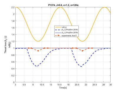
**Figure 5.** Comparison of thrust loss between simulation performed by Dalheim (PropSim(2016)) and Kozlowska (PropSim (2018)) and experimental results of *Koz17*.
