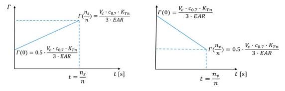
**Figure 7.** Propeller circulation as a function of time to establish the vortex ventilation (top side) and as a function of time for ventilation to dissapear (bottom side),  $K_{Tn}$  is the thrust coefficient for non ventilating condition and  $K_T$  is the thrust coefficient for ventilating condition for given and constant propeller submergence h/R.
