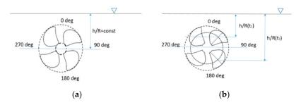
**Figure 10.** Modification of PropSim (2018) in order to account for the effect that the blade thrust loss due to ventilation varies during one cycle of revolution PropSim (2018\_blade\_dynamics). (a) PropSim (2018); (b) PropSim (2018\_blade\_dynamics).
