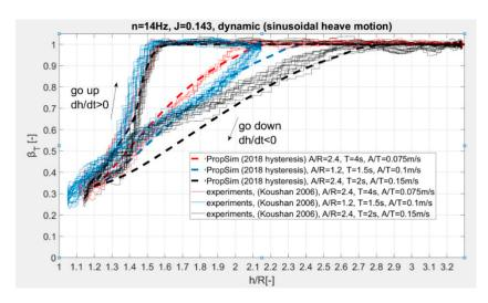
**Figure 9.** Comparison for thrust loss between experiments (dynamic) and simulations (PropSim2018\_hysteresis) for different amplitudes of the propeller (heave), see Case 1, 2, and 3 presented in Table 2, simulation includes hysteresis the effect for two different motions of the propeller (upwards and downwards), PropSim2018\_hysteresis.
