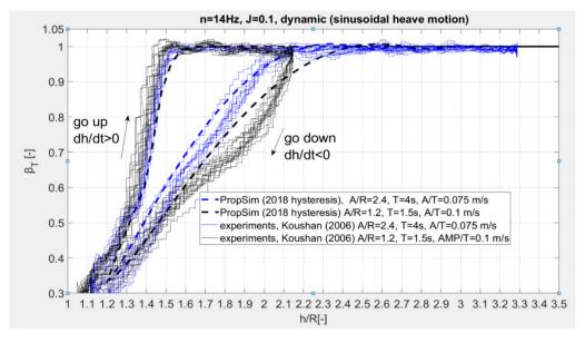
**Figure 8.** Comparison for thrust loss between experiments (dynamic) and simulation (PropSim2018\_hysteresis) for different amplitudes of the propeller (heave), see Case 4 and 5 presented in Table 2; the simulation includes the hysteresis effect for two different motions of the propeller (upwards and downwards), PropSim2018\_hysteresis, the blue line for the up behavior is similar and lies under the black line.
