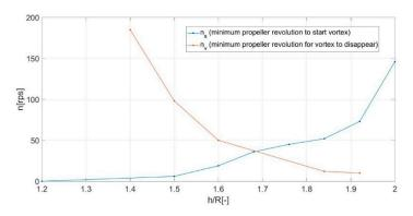
**Figure 6.** Minimum number of propeller revolution to establish a ventilating vortex  $(n_s)$  and minimum number of propeller revolution for the vortex to disappear  $(n_v)$  as a function of propeller submergence, valid only for high Weber number and low advance numbers 0.08 < J < 0.15.
