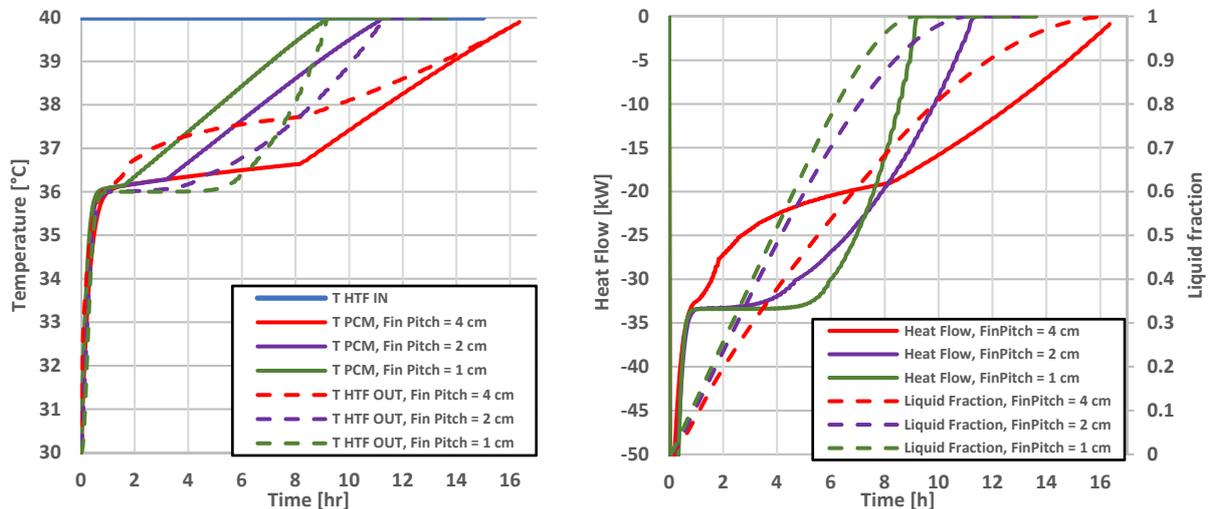
**Figure 4.** Charging process for various fin pitch with constant HTF mass flow of 2 kg/s, (Left) Temperature of HTF at inlet and outlet, and average PCM temperature; (Right) PCM liquid fraction and heat flow from PCM to HTF.
