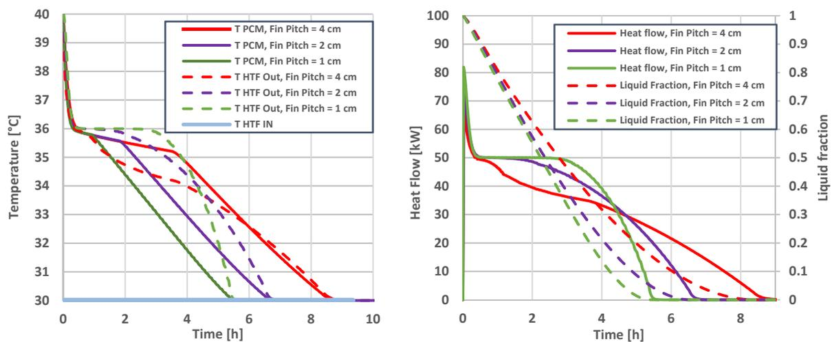
**Figure 5.** Discharging process for various fin pitches with constant HTF mass flow of 2 kg/s, (Left) Temperature of HTF at inlet and outlet, and average PCM temperature; (Right) PCM liquid fraction and heat flow from PCM to HTF.
