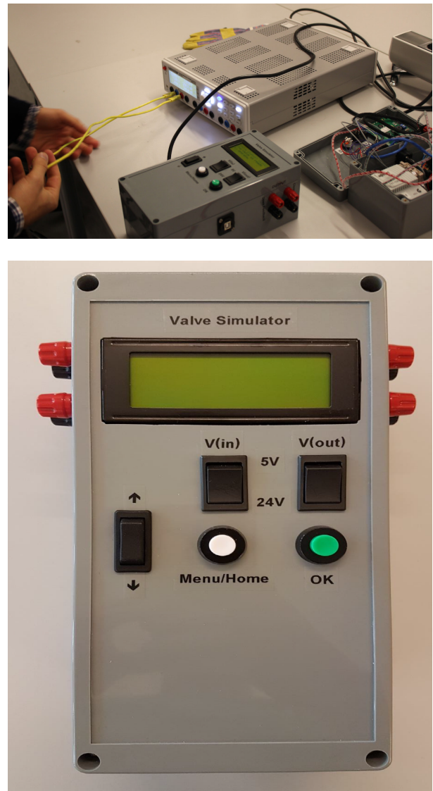
Fig. 2. Development phase (top) and final HIL valve unit (bottom).
