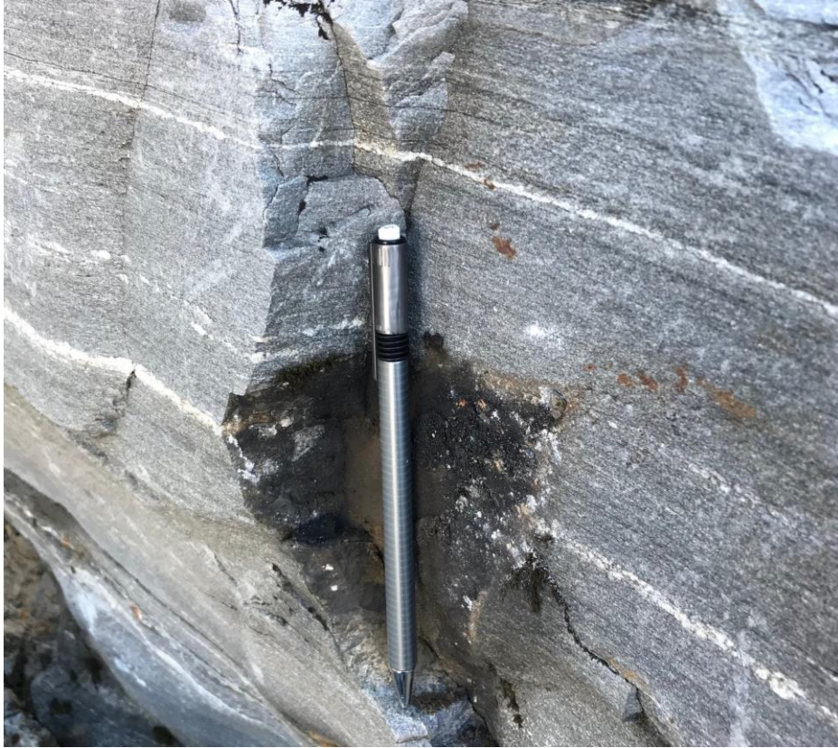
Figure 32. Joint infill location 1.5 in the layer “series 1”. Silty or sandy clay coating. Alternating darker and lighter foliation. The photo is taken towards direction SE (132°).
