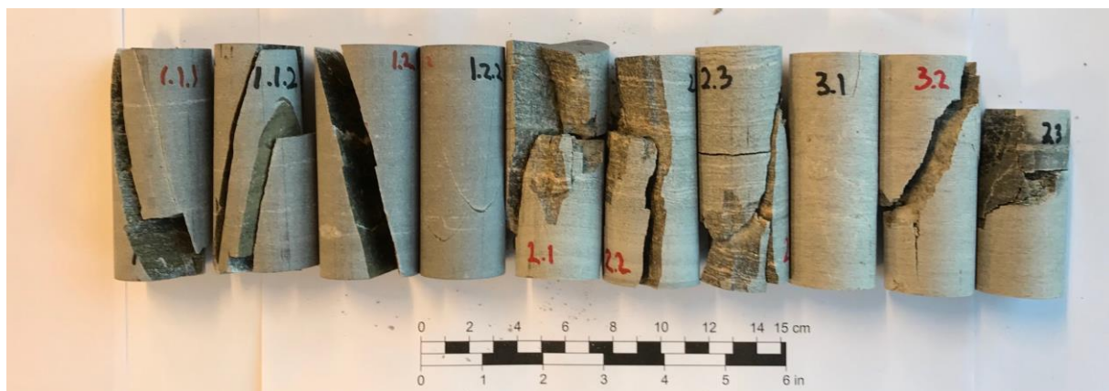
Figure 43. Cores after the uniaxial compressive test.
