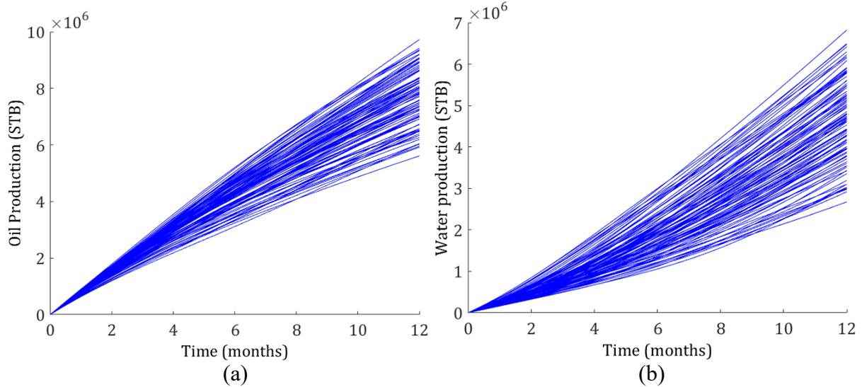
Figure 5: (a) The oil production profiles for all realizations for the first decision alternative, and (b) the water production profiles for all realizations for the first decision alternative.
