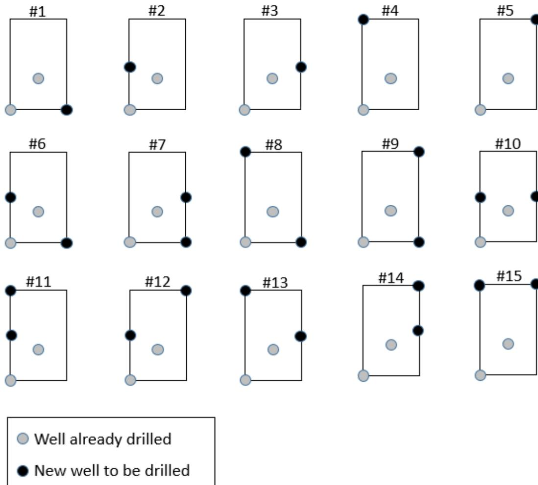
Figure 2: The well locations corresponding to the 15 drilling decision alternatives.
