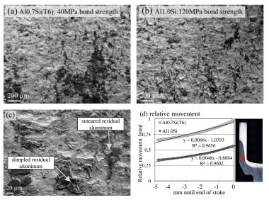
**FIGURE 4.** SEM images of the steel fracture surfaces where the residual aluminum is shown in black for sample joined with Al0.7Si(T6) (a) sample joined with Al1.0Si. Image (b) shows a high magnification of the characteristics of the residual aluminum, smeared or with dimples(c). shows the relative movement at the analyzed position of the highest bond strength(d).
