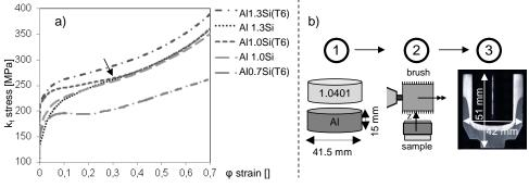
FIGURE 1. Stress stain curve for aluminum materials (a) and process steps (b).
