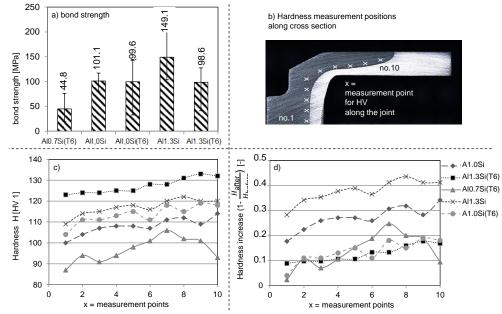
FIGURE 3. Bond strengths (a), hardness measurement positions (b), hardness (c) and relative hardness increase (d) after joining.
