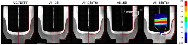
FIGURE 2. Images show the cross-sections of the joined samples with the different aluminum alloys in their different initial states. The red lines show the resulting material flow predicted by the simulations. Right: the contact pressures in the center region are pictured.
