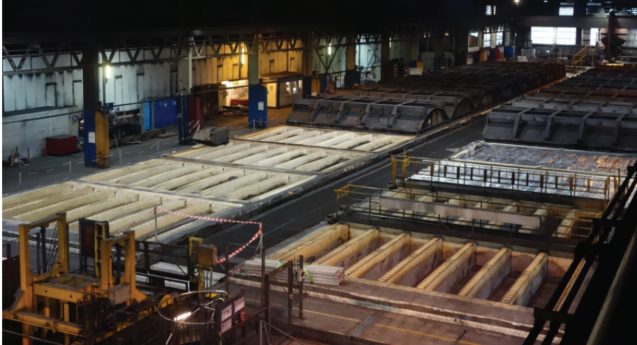
Figure 2.3: The closed top anode baking furnace at Hydro Årdalstangen. Printed with permission from Norsk Hydro.
