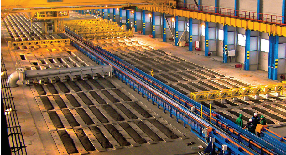
Figure 2.1: The open top anode baking furnace. Reprinted with permission from Riedhammer [46].
