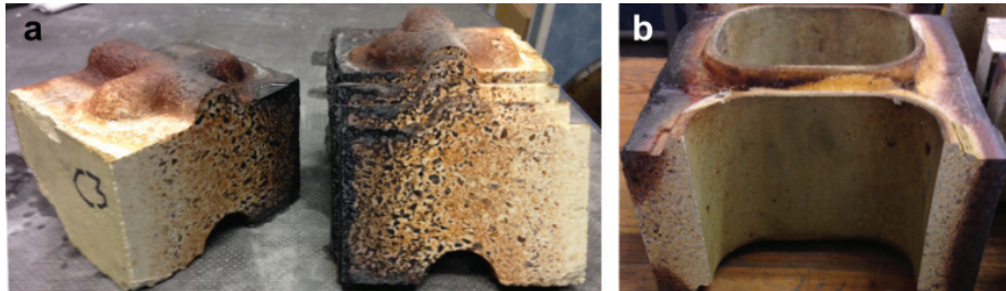
Figure 3.2: Images of the samples taken from a) the open furnace and b) the closed furnace. The pristine refractory material is white/yellow in color, similar as the material close to the flue side. Close to the anode side, the color changes and the spent lining becomes darker and ultimately black in the region closest to the anode side.
