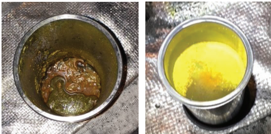
Figure 5.6: Images of pitch condensate in the condensation vessel (left), and discoloring of the white filter material in the filter (right).
