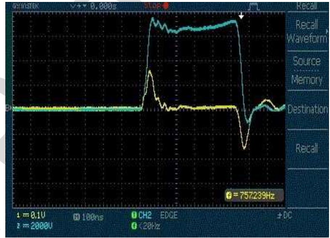
Fig. 20. Typical voltage–current waveform image of LTP Ion mobility system.
