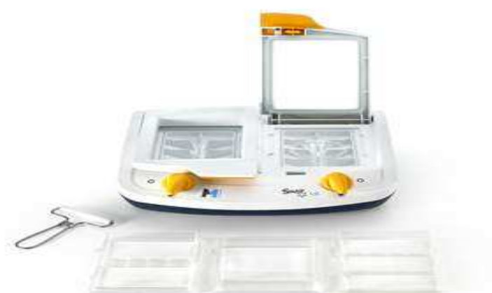
Figure 12: The SNAP id system with the blot holder. This system also consists of a vacuum and a container where all the liquids are collected. This SNAP id is used to incubate the membrane with housekeeping antibodies which takes only 30 minutes (75).
