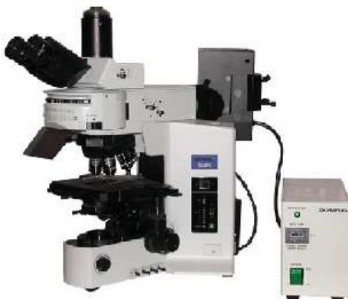
Figure 15 : Fluorescence microscope and different parts. On the left , a picture of fluorescence microscope with mercury-vapor lamp (78). On the right , schematic diagram of the fluorescence microscope with different parts (79).
