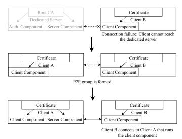
Fig. 2. A client unable to reach the dedicated server establishes a connection with a nearby device. Arrows from the certificates to the client and server indicate authentication during connection.
