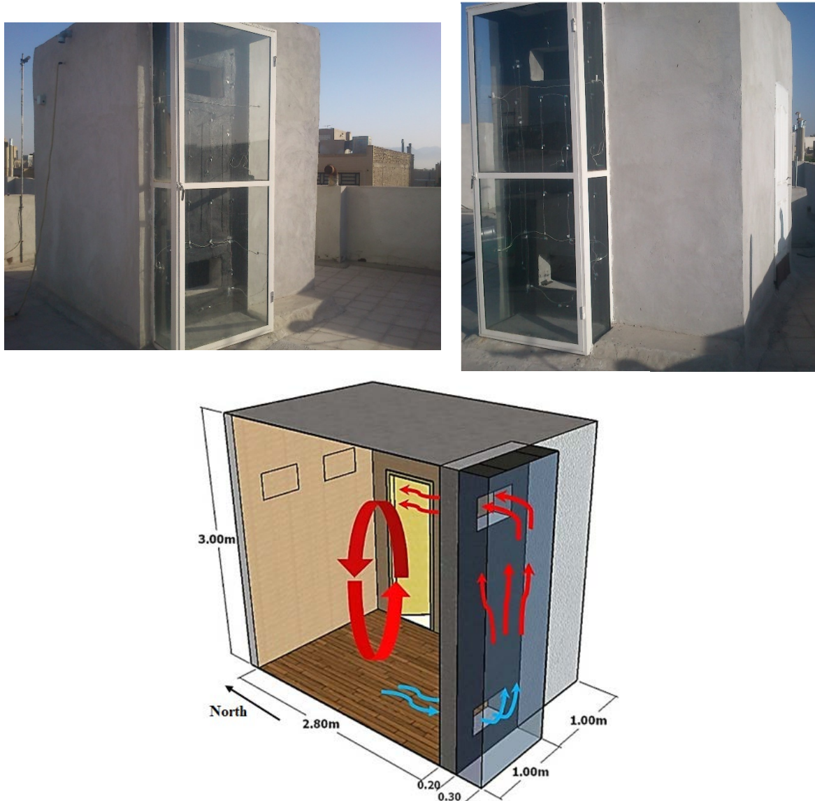
Fig. 2. The new designed Trombe wall and experimental room [23, 24]
