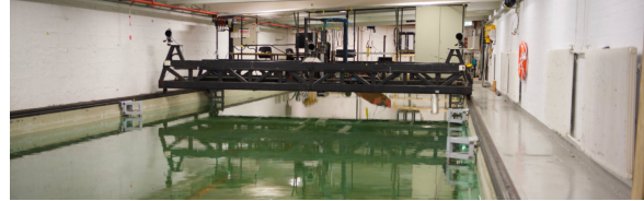
Fig. 8: Water tank in the Marine Cybernetics Laboratory. Dimensions: L x B x D = 40m x 6.45m x 1.5m.
