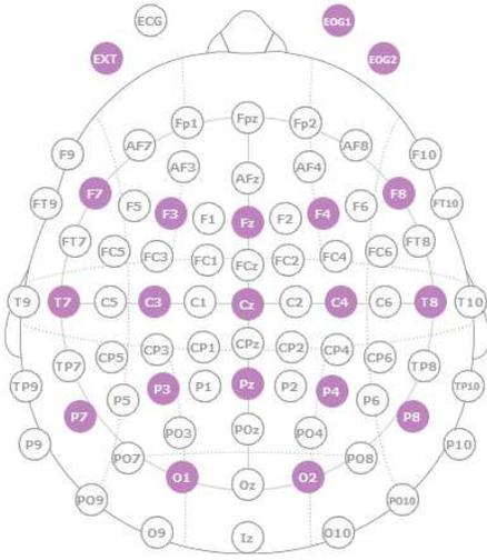
Fig. 3. Electrode layout of 20 channels (17 channels were used for EEG) for the experiment. The coloured ones are the electrodes being used. The white ones are those that the ENOBIO cap provides option for. This is the Standard electrode layout provided by the EEG capturing software. This is also considered as Good all-around montage [41].
