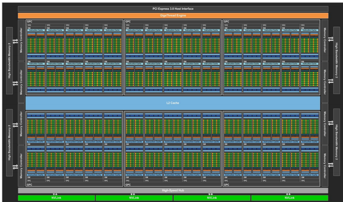
Figure 6: Floor plan of a GP100 GPU taken from NVIDIA 2018(b). We see the 60 SMs, each with 64 single precision execution units and 32 double precision execution units. When a function is run on the GPU it is divided in to thread blocks which are assigned to each SM by a block scheduler (GigaThread Engine). Each SM has a warp scheduler which is capable scheduling two Warps to utilise the 64 single precision execution units represented by the green squares. The 32 double precision execution units are represented by yellow squares.
