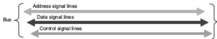
Figure 2. Classification of bus signals [1]
