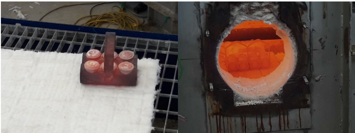
Figure 3-6: Left: First sample holder out of the oven, 10 min. Right: The five remaining samples in the oven.
