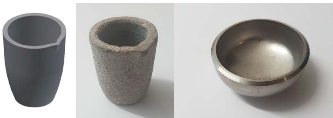
Figure 3-1: Left: Ceram C, the crucible used in 2018 as well as in some of the experiments in 2019. Right: Steel C, the crucible used in the other experiments in 2019.
