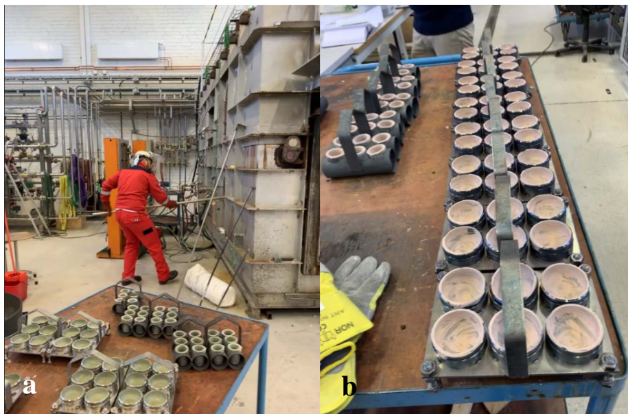
Figure 3-8: Left : The crucibles being set into the oven for drying, Right : The crucibles with dried coating.
