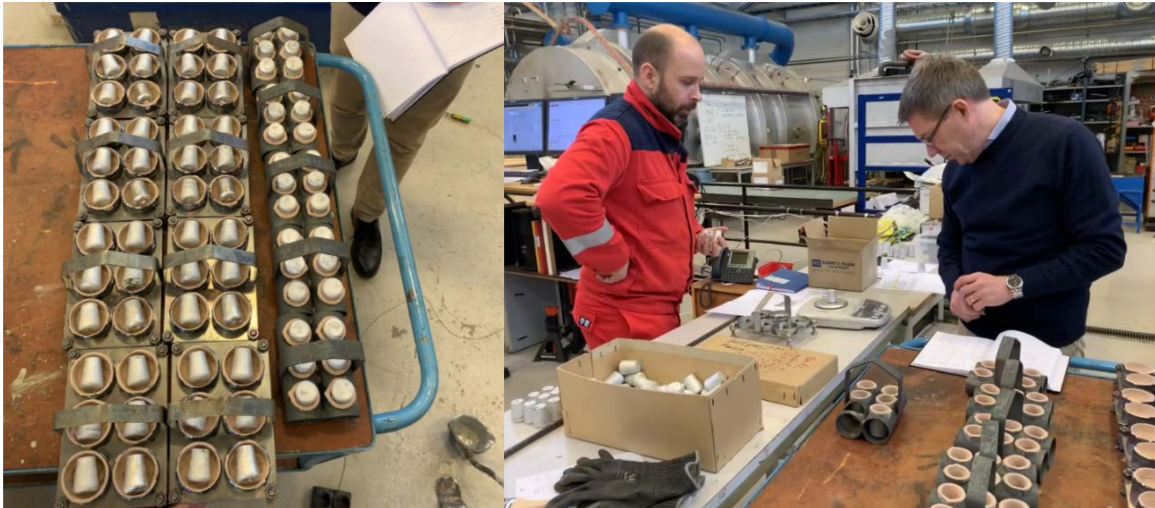
Figure 3-9: Left: Setup with precast alloys. Note that the precast alloys in the steel crucibles have the shape of the ceramic crucible. Right: Weighing the precast samples before the experiment.
