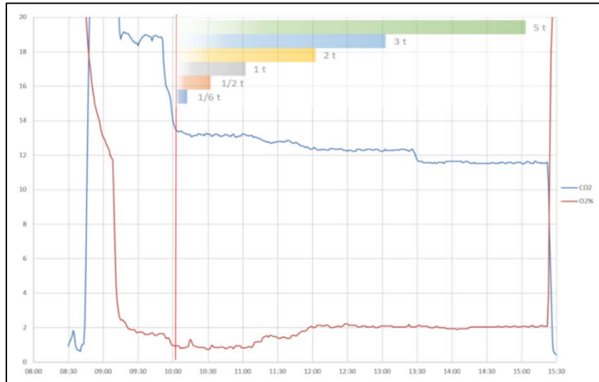
Figure 3-14: Atmosphere 2018, the red line indicates the point in time when the samples melted.
