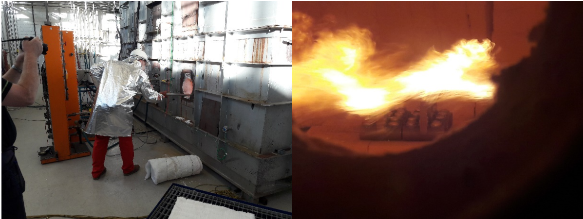
Figure 3-5: Left: The samples being put into the oven. Right: The samples in the oven while gas being burned.
