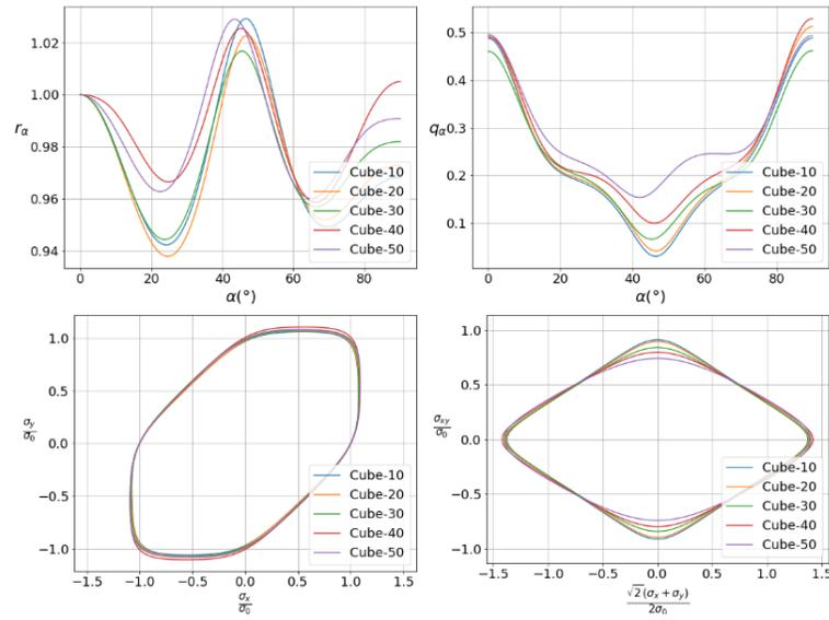
**FIGURE 3.** Normalized uniaxial yield stress, strain ratio and two selected contour plots of the calibrated Yld2004-18p yield function for Cube component, with different ratios of random component.
