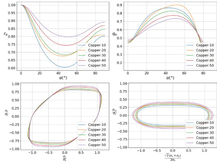
**FIGURE 4.** Normalized uniaxial yield stress, strain ratio and two selected contour plots of the calibrated Yld2004-18p yield function for Copper component, with different ratios of random component.
