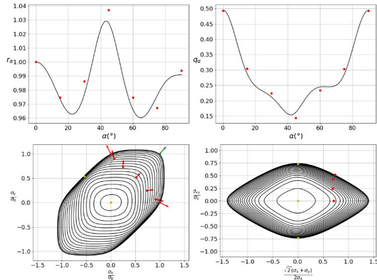
**FIGURE 2.** Normalized uniaxial yield stress, strain ratio and two selected contour plots of the calibrated Yld2004-18p yield function for Cube component with 50% randomness.
