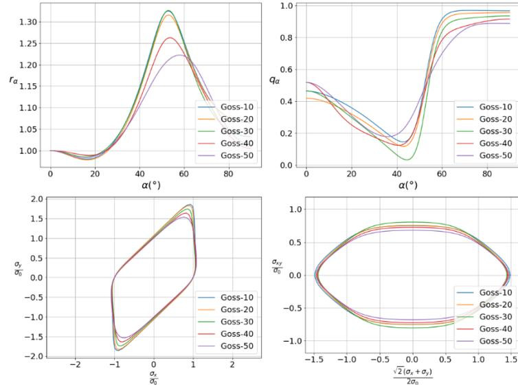
**FIGURE 5.** Normalized uniaxial yield stress, strain ratio and two selected contour plots of the calibrated Yld2004-18p yield function for Goss component, with different ratios of random component.
