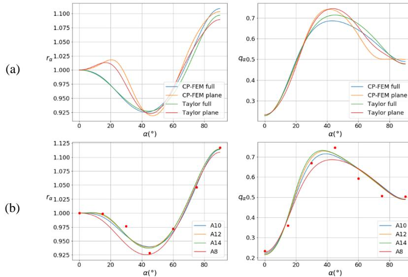
**FIGURE 6.** Normalized uniaxial yield stress and strain ratio for Brass component with 50% random component using (a) different homogenization and calibration approaches, and (b) for different values of the yield function's exponent.
