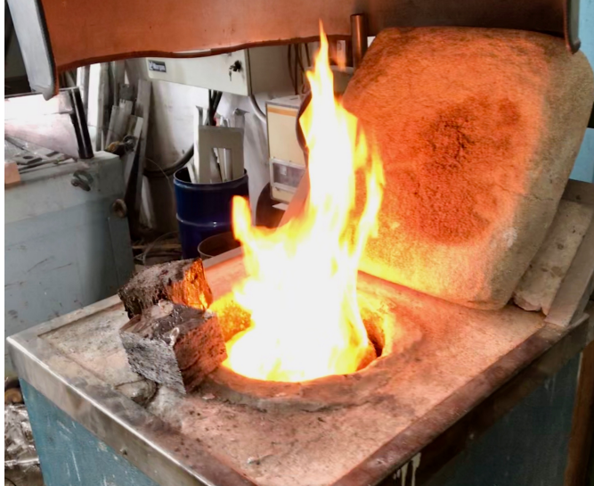
Figure 5.21: Combustion of flammable gases released from Cans 300 during remelting.
