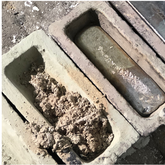
Figure 6.9: The chamotte-colored bottom dross cleaned out of the crucible after decantation of melt from experiment 7.
