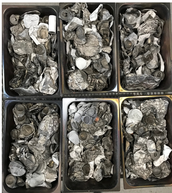
Figure 5.12: Cans sample material decoated at 550 °C - Cans 550 . In thee middle we see a white porous material deposited on the side of the trough surrounding sample material.
