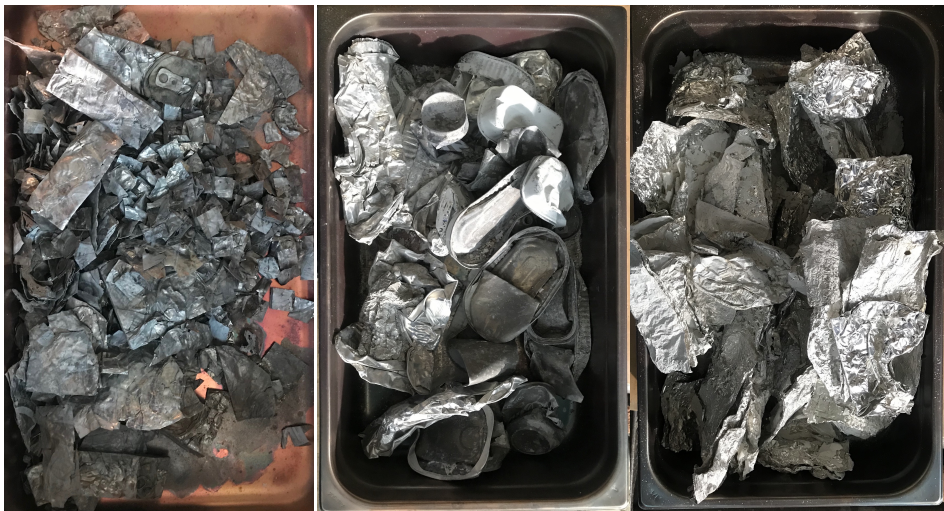
Figure 5.2: Preliminary: UBC (left), Cans (middle) and Foils (right) after heat treatment
