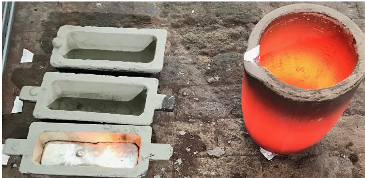
Figure 5.4: Sample of remelted cans next to still molten crucible.
