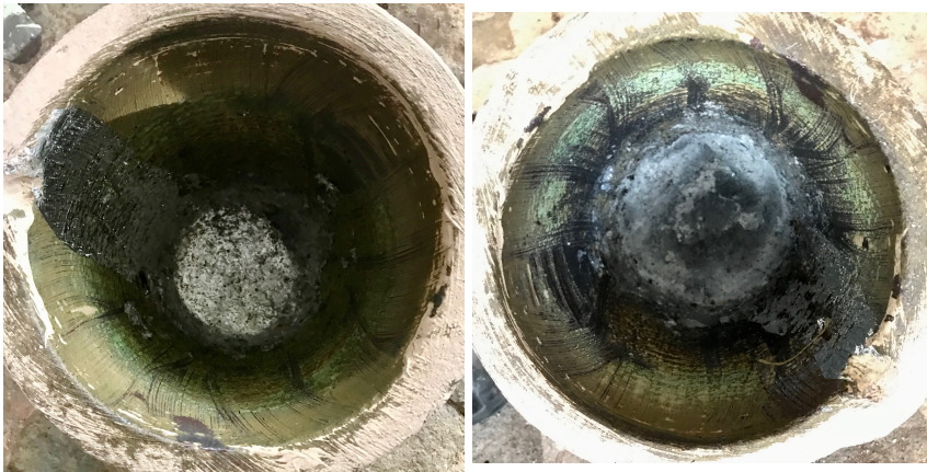
Figure 5.6: Empty crucibles after remelting Cans (left) and Foils (right). The left crucible contains a sheet of metal whilst the right crucible contains bottom dross.
