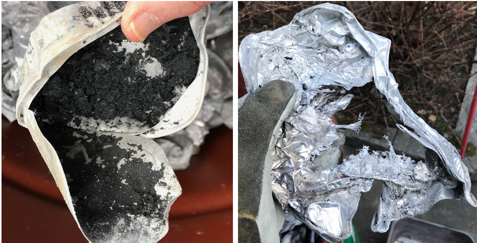
Figure 5.7: Examples of sample pieces from Cans 550. A partly opened canned food can filled with black char (left). A partly disintegrated aluminium tray (right).
