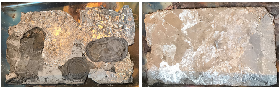
Figure 5.3: Preliminary: Cans (left) and foil (right) after compaction
