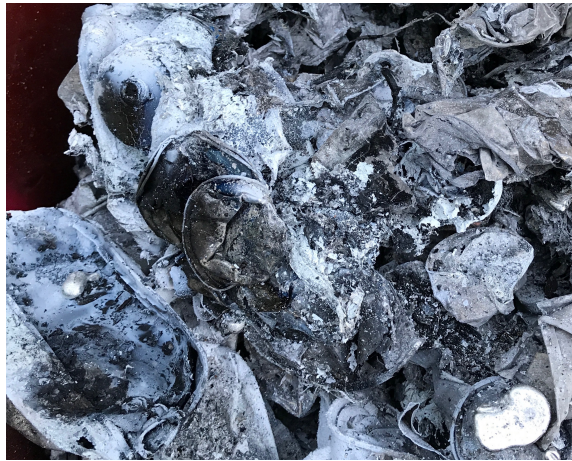
Figure 6.2: The contents of a large trough of Cans decanted at 550 °C flipped over. The material seems to be covered in metal oxides.
