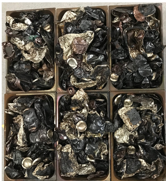
Figure 5.11: Cans sample material decoated at 300 °C - Cans 300
